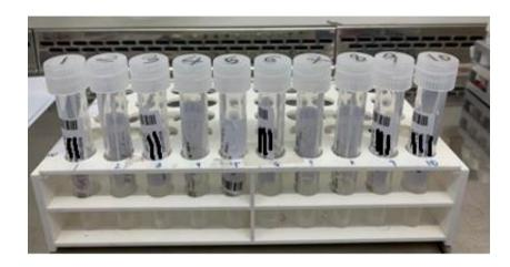
6. To avoid sample hazard leak and label fading, keep the rack in a zip-lock nylon bag surrounded by absorbent material.
